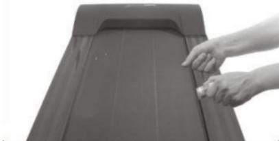
Pull up tightly of the running belt. Then put the silicone oil to running board. Then start the machine to running 3 minutes without loading. It is better to maintain like this every 30 hours working of the machine. This can save lifetime of parts properly.
