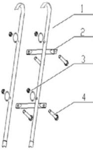
Install the ladder, connecting components with bolts and nuts included in the assembly kit.
