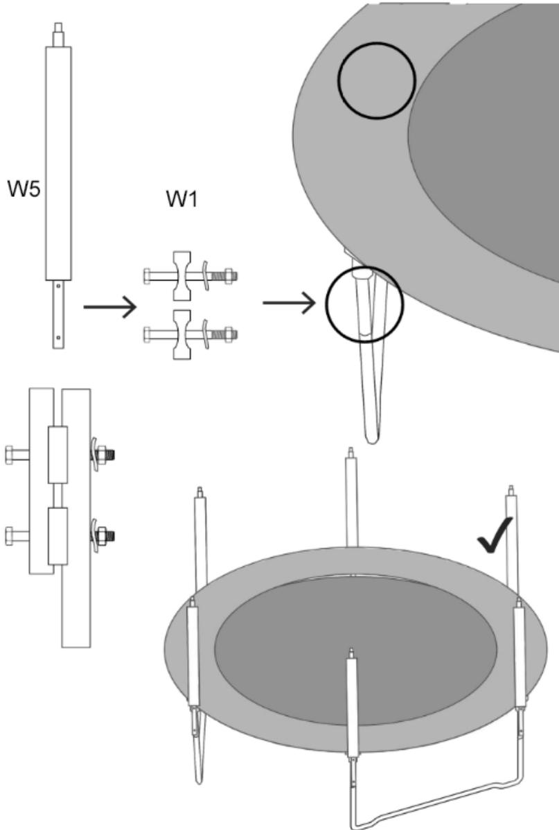
At this assembly stage the trampoline should look as shown in the above figure.
