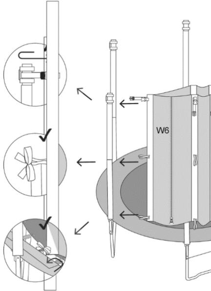
**PLEASE NOTE:** Ensure all mesh fastenings are installed correctly and are tight.
