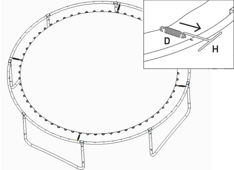
To ensure uniform bed stretch, attach the springs alternatively on 4 sides of the frame. Install the first one at 12.00 of the frame, the second at 6.00, the third at 9.00 and the fourth at 3.00. The successive springs should be installed analogously at four sides of the frame.
