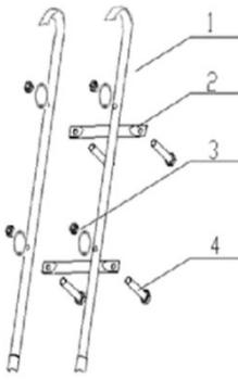
Install the ladder, connecting components with bolts and nuts included in the assembly kit.
